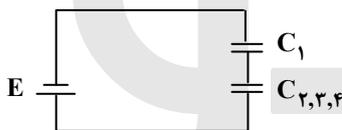
$$q_1 = q_{2,3,4} \rightarrow C_1 V_1 = C_{2,3,4} V_{2,3,4}$$
